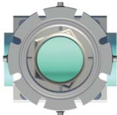
Figure 8 Completion pins NOT flush with inner valve flange. DO NOT ATTEMPT VALVE INSTALLATION WITH PINS IN THIS POSITION.
